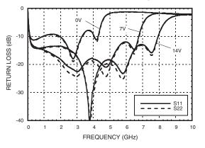
Return Loss vs. Temperature, Vfctl @ 7V [1]
