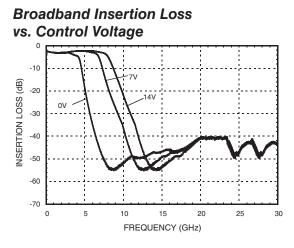
Insertion Loss vs. Control Voltage [1]
